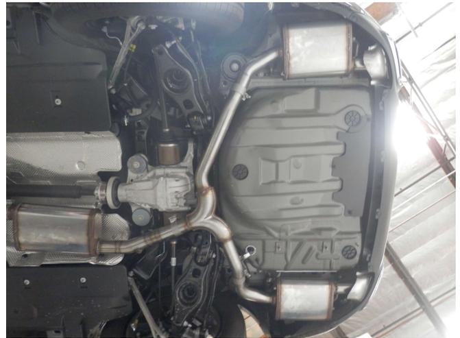
**Step 4.** Install the Y-Pipe Assembly, drivers and passengers side Muffler Assemblies in a similar fashion using the supplied 2.50" clamp. Locate each muffler outlet to each OEM tip mounted in the vehicles valance. Engage the welded hanger to the OEM rubber insulators.
